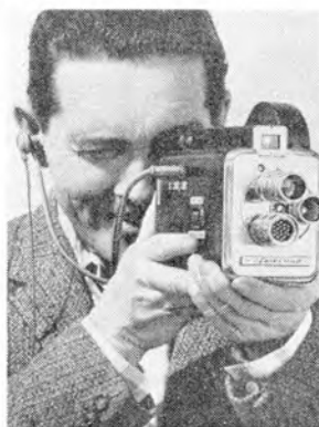
Left: The world's first 8mm single system camera, photographing and recording on one piece of pre-stripped film. A transistor recording amplifier is built into the camera body, and headphone monitoring is provided. The Fairchild Cinephonic 8 camera takes 50 ft. reels of double 8 film, and costs £185. On the right is the camera's matching unit, the Cinephonic 8 projector. This allows additional sound to be added to the track which has already been made in the camera. The price is £185
